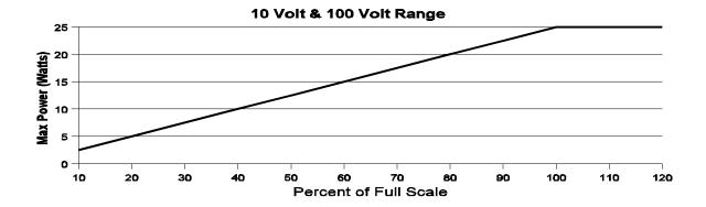
Maximum power output is proportional to the output voltage expressed as a percent of full scale, and is  $\sim 25$  watts at 100% of range.
