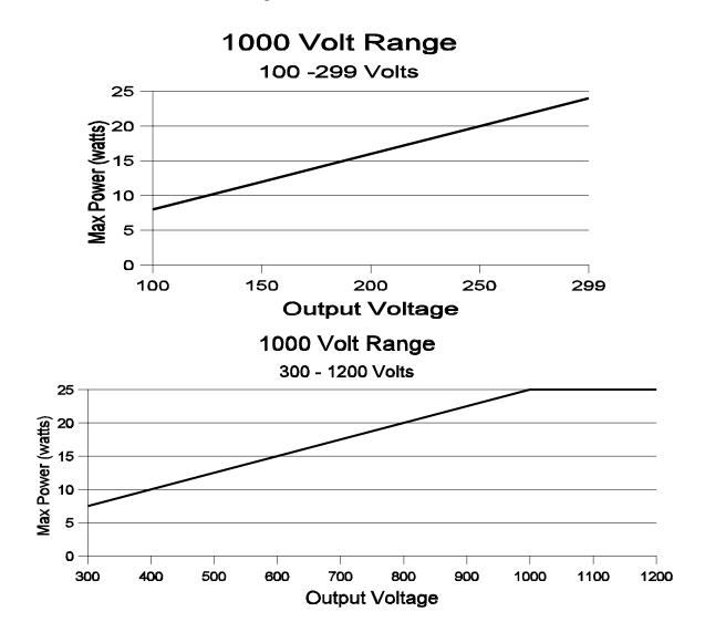
Maximum power is proportional to output voltage up to a maximum of  $\sim 25$  Watts. On the 1000V range, the output transformer taps are switched at 300V. The maximum power output varies between 8 and 25 watts between 100V and 299V, and again between 300V and 1000V. On the 1V range the maximum current is 1Amp. Therefore, the power output at 1V = 1 Watt, and at 0.1V, it is 0.1 Watt. The 100mV range is a divided output, with 10 Ohms
